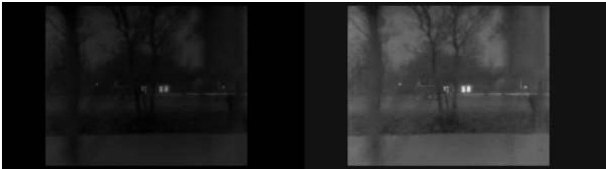
*Boat at 2km and house at 3km Virtual Iris™ protecting the tube and ShadowBoost™ improving the contrast. ShadowBoost™ activated on the right. Recorded during overcast dusk with 600mm Nikon f4.0 lens connected to Pulsatrix™ camera.*
