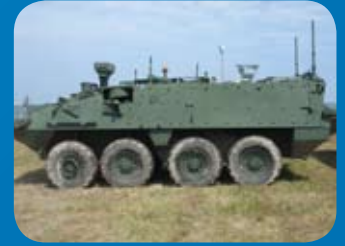
Omni antennas on armoured vehicles
