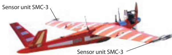
MDI AS-113/12U installed in the ALBA target
