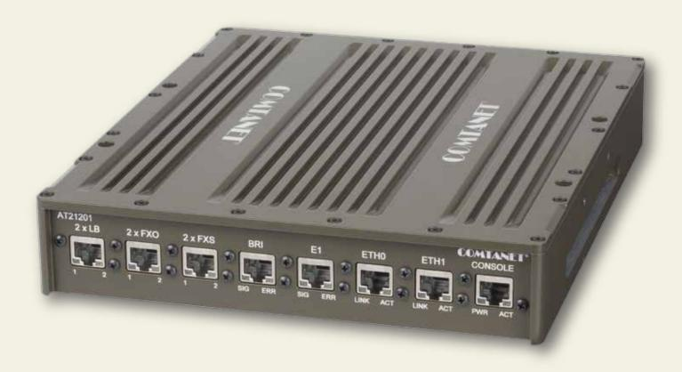
AT21201 Voice Communication Gateway (VCG) provides a voice gateway between VoIP networks, legacy and radio networks. The VCG enables switching a radio from receive to transmit (PTT function) as well as setting up the basic para-meters of the radio, from an IP phone (channel, operation mode, selective dialing, etc.)
