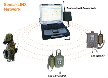
Sensar-LINX wirelessly integrates LCD 3.3 and LCD-NEXUS detectors.
