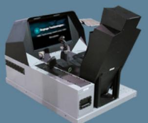
MRC shown with Bugeye simulated ejection seat and long-throw center mounted stick. Full length Dzus rails to locate simulated throttle position and support additional console mounted equipment. The MRC supports center stick and side-stick configurations.
