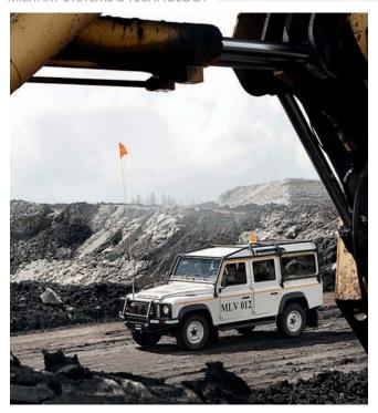
For safety around the mine environment they are fitted with amber roof lights, reversing buzzers, top and bottom reversing lights, and a flag pole mount. The latter provides improved visibility when operating in the vicinity of larger mine vehicles. An option is a roof-mounted LED light bar that can be programmed to display signals to drivers of other vehicles.
