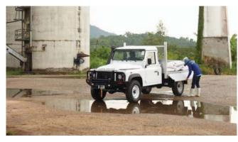
fitted to any AVM Defender. The 110 series, for example, can be fitted with enhanced suspension to raise gross weight to 3500kg. A winch with a 4500kg capacity can be installed in either 110 or 130, as can a rear towing hook for towing. Fuel consumption will vary from one product to another, determined by the type of conversion undertaken.
