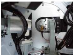
polarization duplexers which separate or combine transmit and receive signals. The common circular waveguide port with a standard diameter of 19.05 mm (= 0.75") is used as antenna port which carries both transmit and receive signals by means of two orthogonal H11 modes.
