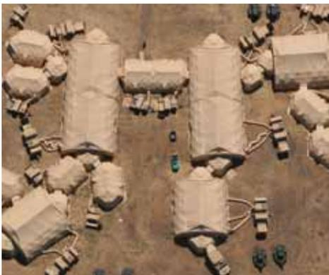
product, the Deployable Rapid Assembly Shelter (DRASH). DRASH is a quick set-up/strike soft walled shelter specifically designed for mobility and rapid deployment. DRASH Shelters come in a variety of makes and models, fulfilling the diverse needs of its customers.
