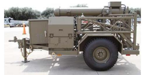
Dewey Electronics and its partners, Essence Solar, Silver Eagle Manufacturing Company, and EnerSys, have produced a demonstration hybrid platform that incorporates solar generated electricity, an integrated backup military tactical generator, and battery storage all on a standard Lightweight Tactical Trailer (LTT). This system features a patent pending dual axis solar tracker with High Concentration Photo Voltaic solar panels that provide 25% more solar power than standard flat solar panels.
