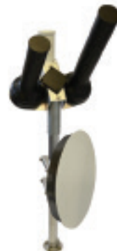
Counter-UAS antenna array
