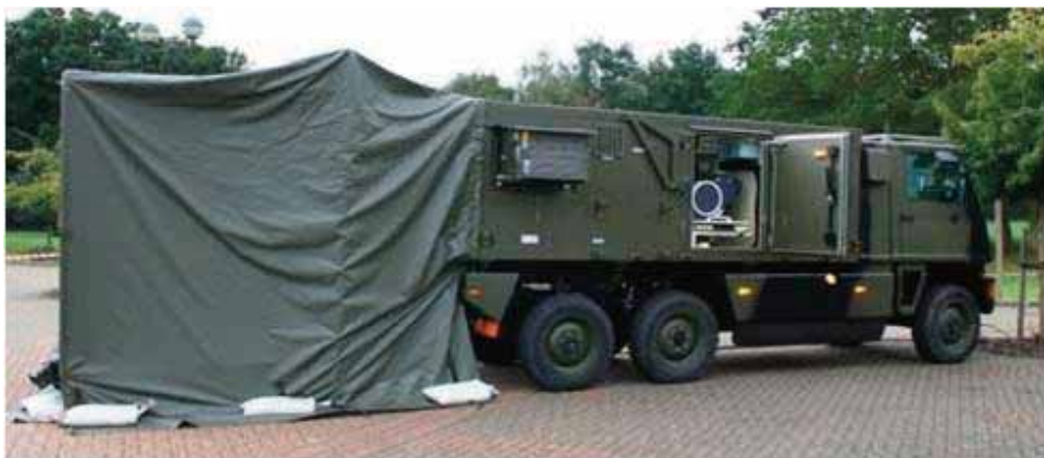
Marshall Land Systems as part of Team SOCRATES has integrated GEOINT analysis equipment and printers into shelters fitted to the MOWAG Duro II 6x6 vehicle.
