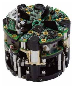
Available interfaces: Full speed USB2, RS232/485-422, Ethernet LAN and SPI.
