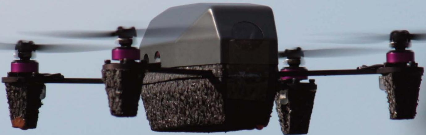
"The drone can be flown remotely using a tablet, which also displays the video and stills transmitted by its high-resolution camera. Its small size coupled with its 10 ultrasonic sensors make it ideal for penetrating and searching buildings and narrow spaces. It can hover discreetly over a targeted area or 'perch and stare' using day or night vision.
