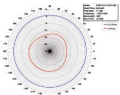
Radiation Pattern -Elevation. At the centre frequency of 1.087GHz, this pattern shows 1.5' electrical up-tilt and 17' elevation beamwidth
