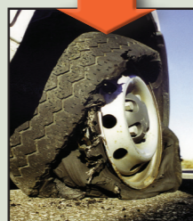
As a deflated tyre collapses, the wheel rim can come into contact with the road causing loss of control
