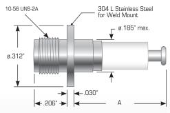
Series 600 "S" A = .550 max Series 600 for welded & solder flange installation A = .520
