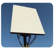
HBS - Hub Base Station Multi-Beam antenna can provide 90° azimuth coverage in two polarisations from six high gain beams. Four Hub Base Stations are used at a central location for 360° coverage. The HBS communicates with a network of Hub Subscriber Stations (HSS).
