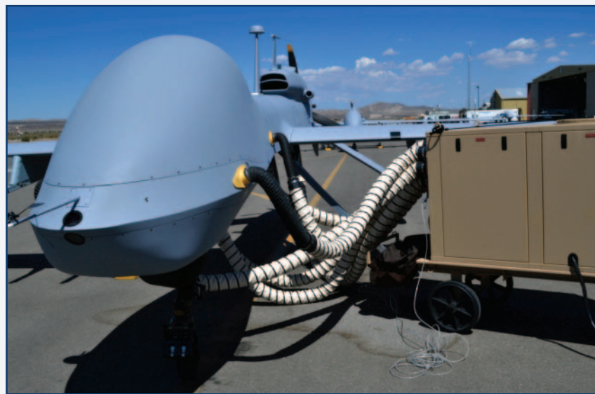
A DRASH 5-ton ECU cools a Gray Eagle aircraft vehicle prior to flight.
