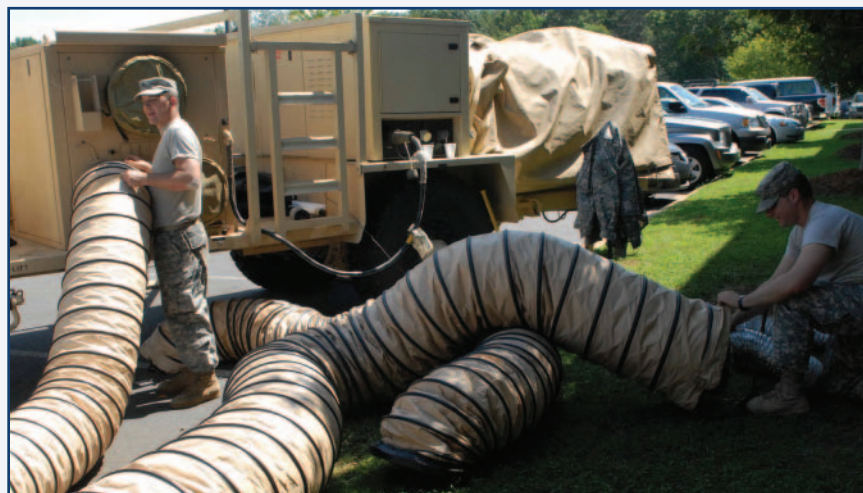
Guardsmen set up DRASH ECUs to provide air conditioning for their Joint Task Force mission.
