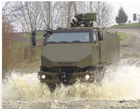
Duro IIIP powered by ISBe 5.9 245 hp (Mowag)
