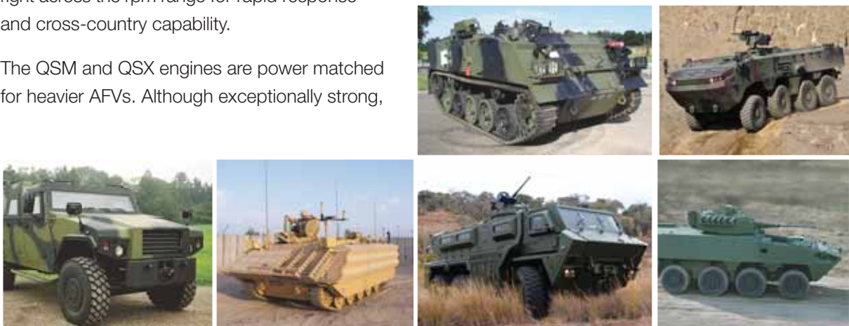
Clockwise from top: British Army FV430 MK3 powered by 6BTAA 250 hp (BAE Systems), ARMA 8x8 armoured vehicle powered by ISLe T450 hp (Otokar), Portuguese Army Pandur II 8x8 AFV available with ISLe T450 hp (Steyr-Daimler-Puch), the RG-35 is a multi-purpose mine protected armoured vehicle, powered by an ISL 450 hp (developed as a private venture by BAE Systems in South Africa), British Army Bulldog upgraded armoured fighting vehicle powered by 6BTAA 250 hp (BAE systems), Danish Army Eagle IV Armoured Patrol Vehicle with ISBe 250 hp (Mowag)
