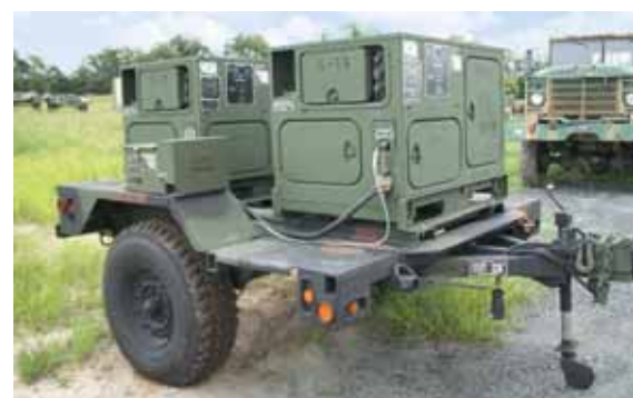
The Advanced Medium Mobile Power Sources (AMMPS) for on-site power generation
