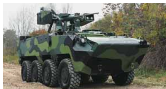
Czech Army Pandur II 8x8 AFV powered by the ISLe T450 hp (Steyr-Daimler-Puch)
