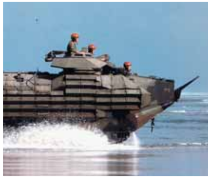
Left: US Marine Corps AAV7A1 Amphibious Assault Vehicle powered by the V903 (BAE Systems) Right: British Army, 155mm AS90 self-propelled howitzer, equipped with VTA903 T660 hp (BAE Systems)
