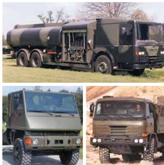
Clockwise from top left: UK Royal Air Force 6 x 4 aircraft refueller designed for air transportability, powered by a 245 hp C Series (Dennis Eagle), Duro III military tactical vehicle 6x6 powered by ISBe 185 hp (Mowag), High mobility 6 x 6 tactical truck powered by an ISM 400 hp (ATC/TATRA)
