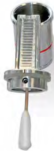
Sample container using a cotton bud for taking liquids.
