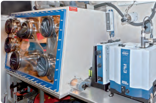
Mass spectrometer and gas chromatograph E2M for detection of substances in soil, liquid, air and on surfaces.
