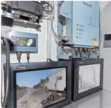
Ion mobility spectrometer RAID-S2 for detection of chemical warfare agents and toxic industrial chemicals in the environmental air.
