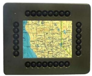
The 29LMV Series of LCD monitors have been designed to comply with military specifications to make it suitable for use within vehicles and areas where shock and vibration are key criteria.
