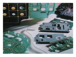
The choice of LED's in a Surface Mount configuration enables panels for Aerospace and Military applications to be manufactured in accordance with the requirements of MIL-DTL-7788G (Formally SAE AS7788) for Type VII panels.
