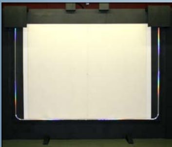
Live-fire screen with high-speed bullet- tracking sensors
