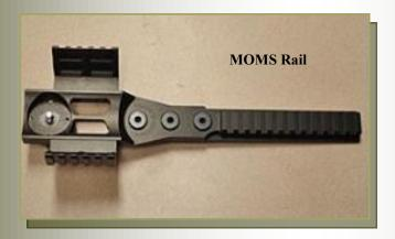
MOMS was designed for the needs of special observation groups. It allows the Spotter and shooter to view the same target simultaneously. The mount is specifically designed for the Leupold Spotting Scope and allowing for the fitting of front mounted NV or TI units It is machine cut from a solid block of aircraft grade aluminum resulting in light weight, but very high strength. There are two wings mounted left and right for accessories such as lights and lasers.
