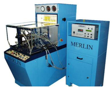
Suitable for testing Bosch CP1, CP1H, CP1K, CP3, Delphi, Denso and Siemens systems
