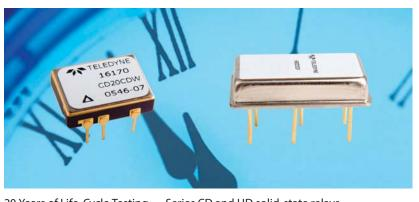
20 Years of Life-Cycle Testing — Series CD and HD solid-state relays have undergone 105,000 hours of permanent testing without a single failure. That's the equivalent of 376 million cycles. Test conditions featured a full load at 50% duty cycle, 85°C ambient temperature and V-load = 60 Vdc. The test parts met all given specifications.
