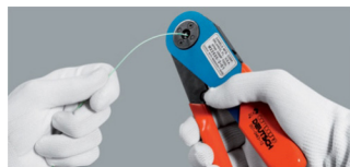
STEP 5: Tighten the crimping tool.
