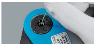
STEP 4: Insert the wire in the contact.
