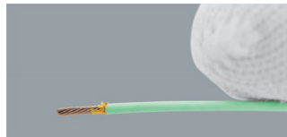
STEP 2: Strip the insulation* 5 mm maximum.
