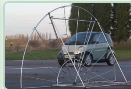
Semi-circular array used for moving source beamforming
