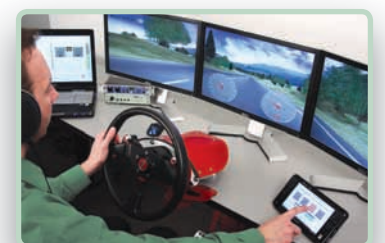
NVH desktop simulator helps you evaluate the sound before you build the vehicle and design the sound of the vehicle to meet brand and customer expectations
