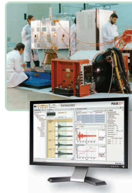
Satellite vibration and shock testing with LDS V984 vibration shaker and PULSE Reflex Shock Response Analysis
