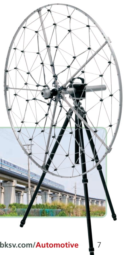
Moving source beamforming used to pinpoint noise sources on high-speed trains
