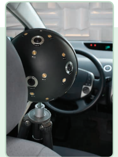
Spherical Beamformer used for in-vehicle measurements
