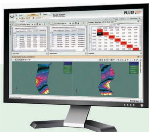
PULSE Reflex Modal Analysis is a modern and intuitive application for classical modal analysis, being used here for aircraft engine turbine blade testing
