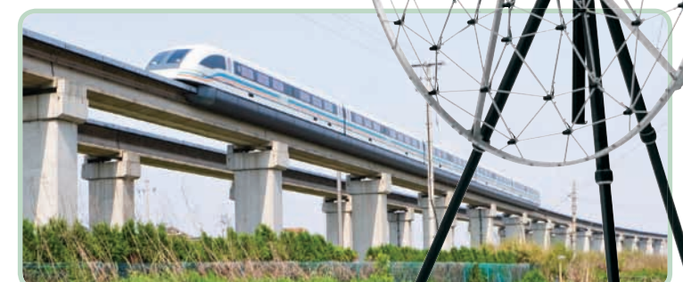
Moving source beamforming used to pinpoint noise sources on high-speed trains
