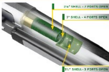
SELF-REGULATES GAS PRESSURE BASED ON THE LENGTH OF THE SHELL FOR FLAWLESS CYCLING OF ALL LOADS.
