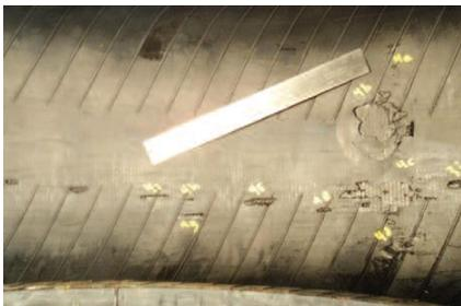
Secondly, rubber is a compliant material and prevents the damage caused to the tyre from impingement between the runflat and the inside of the tyre. The tyre manufacturers have sent out circulars with regards to these problems.
