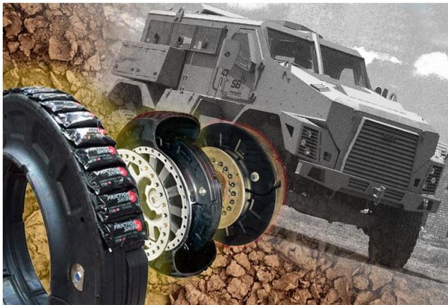
In 2009 Tyron developed the unique R series wheel for armoured 4x4, 6x6 and cash carrying vehicles. This super strong alloy wheel, with a load rating of 1650kg, incorporates an ingenious beadlock design. When fitted with the ATR they allow travel on or off road for over 50km with all tyres deflated.
