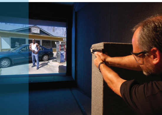
ShootBack cannon synchronises hostile return fire with the shots fired by the actor on the screen
