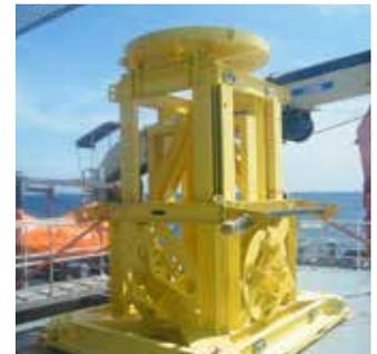
500m rated 60° capable mating target. Transportable in 10' ISO container
