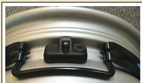
Special TPMS brackets are available to fit around wheel sensors if you have a Tyre Pressure Monitoring system fitted.
