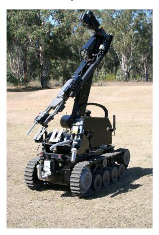
The tEODor is the only vehicle in its class that has three tool magazines integrated in the chassis. This means that up to three additional tools or weapons can be carried in an operation, eliminating the need to return to the base station in order to pick up new equipment. The user saves valuable time, permitting him to
