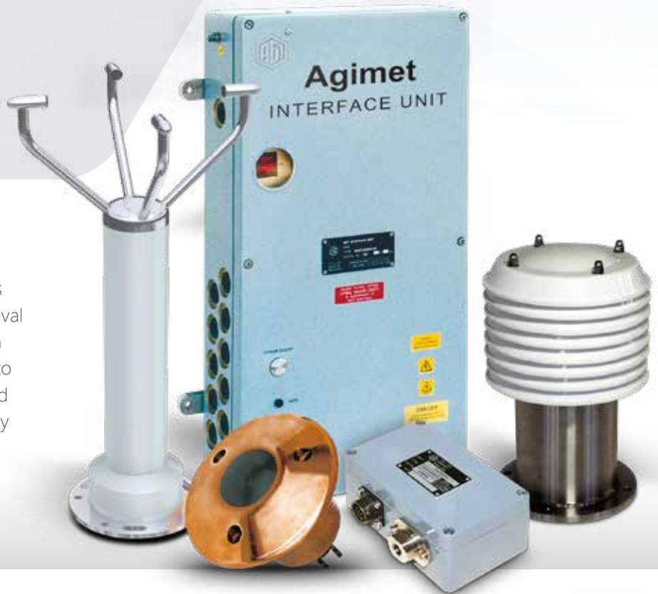
A typical ships system will comprise two solid state wind sensors - mounted port and starboard together with additional meteorological sensor options, each sending data via an interface unit to solid state displays and other systems. Information is transmitted digitally, simplifying data handling and alleviating the need for dedicated re-transmission. Wind outputs from the windward sensor are monitored continually by the AGIMET Interface Unit
