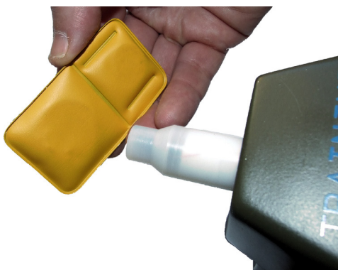
Simulation Point Contact Sources (PCS) for decontamination training
