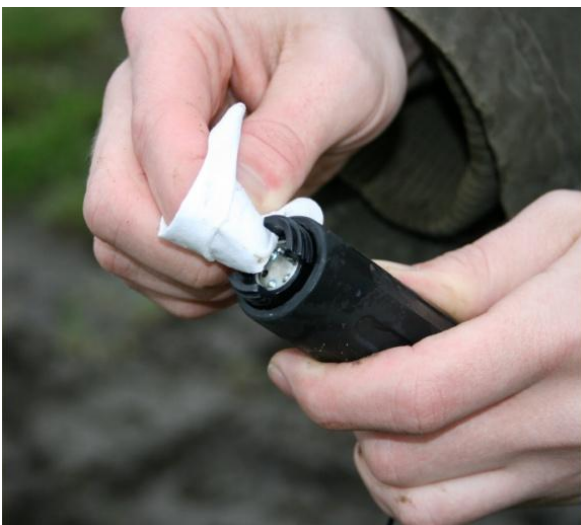
5. The insert face is dried and wiped clean. Ideally a clean cloth or tissue is used but if these are not available the bottom of your coat will suffice. No damage to the insert surfaces or lenses will occur.
