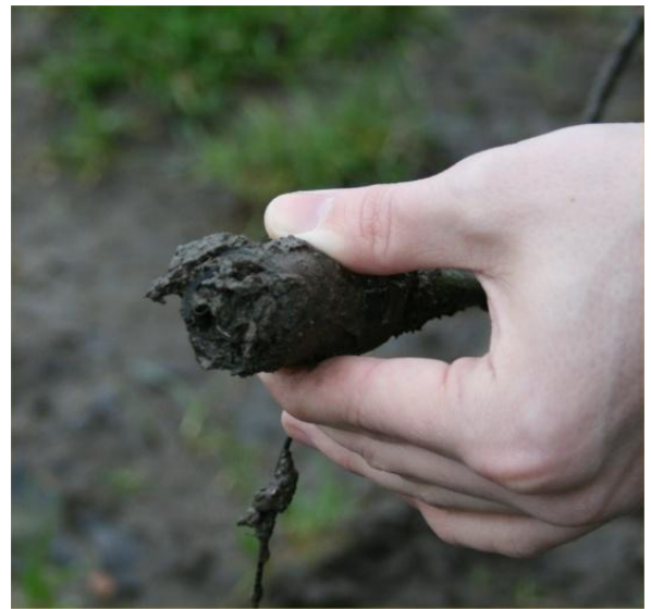
2. The mud will not cause damage to the insert. A physical contact connector would almost certainly already be destroyed in this state.
