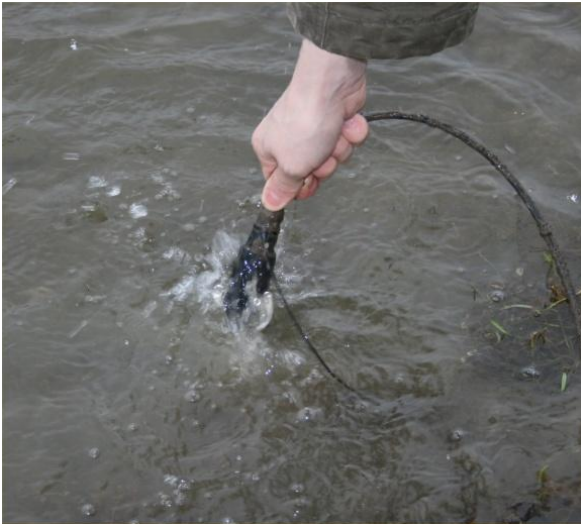
3. Initial cleaning to remove mud and debris from the connector face can be done by rinsing in water. A hose, bucket of water, stream or muddy puddle will do.
