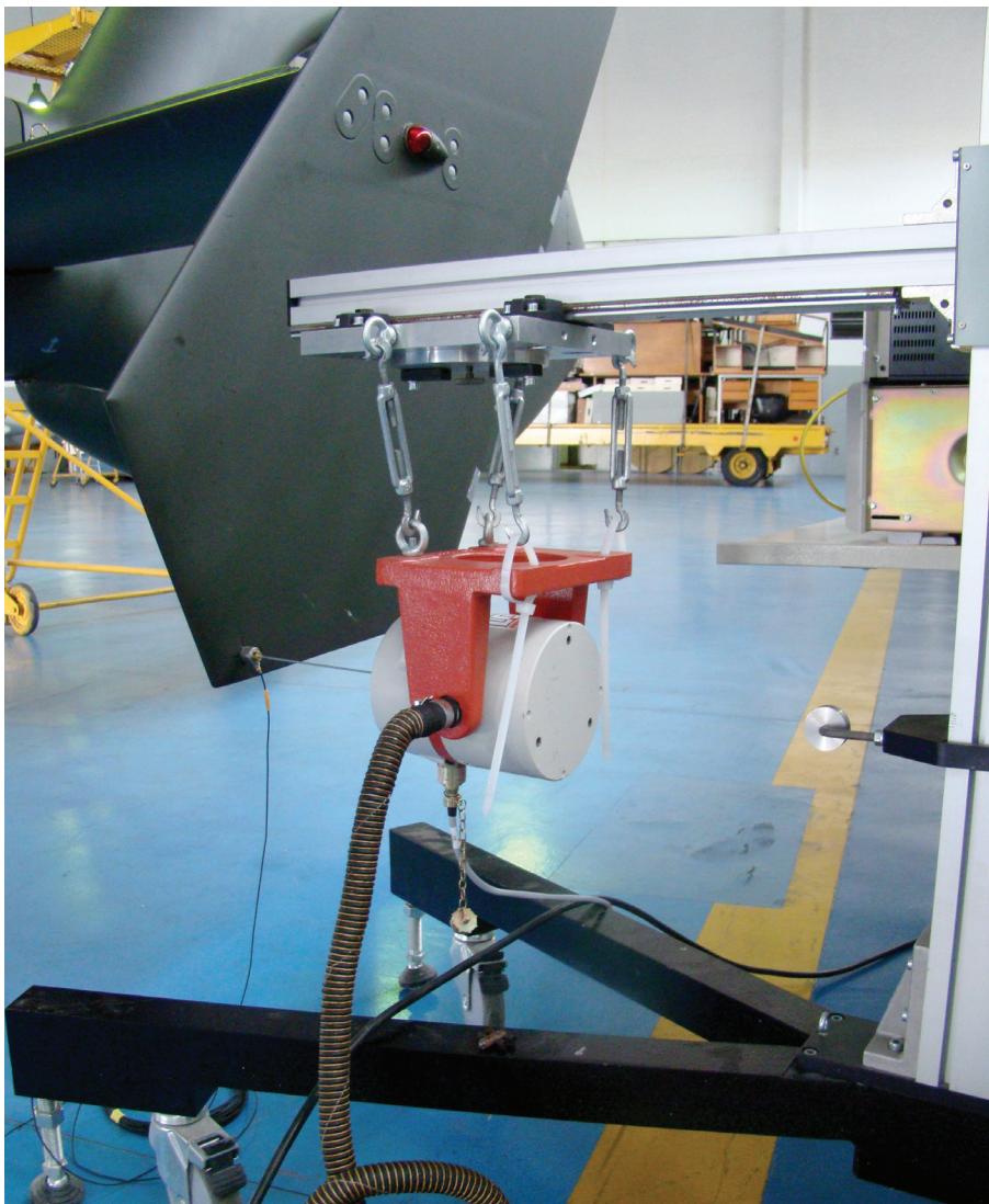
On-ground testing to identify critical modes used a combination of an LDS V455 shaker, and a Brüel & Kjær Heavy Duty Impact Hammer Type 8207 for excitation
