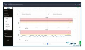
GIDAS, developed by OHB Digital Solutions, is a scalable real-time GNSS Interference Detection & Analysis System, used as a standalone monitoring station for interference detection and classification. The system can be upgraded to a more complex network of standalone stations, which allows interference localization in addition.
