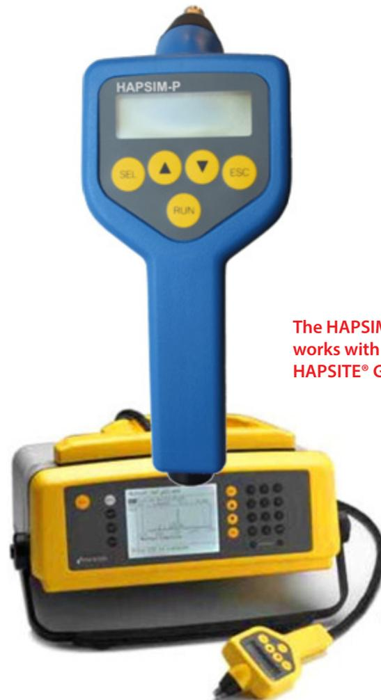
**The HAPSIM-P probe works with the real HAPSITE® GC/MS.**
