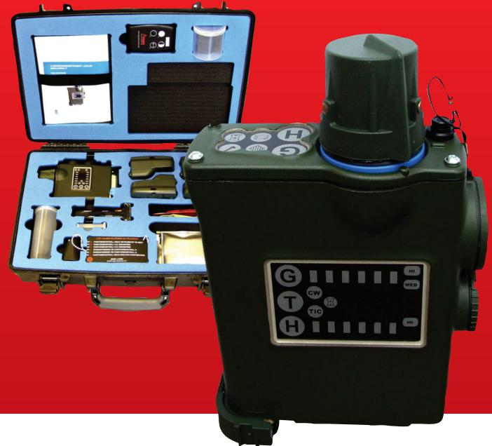
**The JCAD-SIM detector simulator responds to electronic sources that simulate chemical vapors, toxic industrial substances or false positives.**
