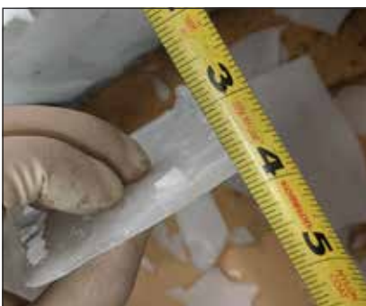
The Night Scan Powerlite IQ was tested at -26°C (-15°F) with 6mm (1/4") of ice
