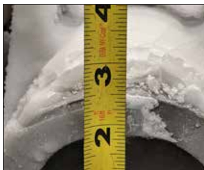
The Night Scan Powerlite IQ was tested at -26°C (-15°F) with 6mm (1/4") of ice
