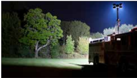
Dual optics for near and far illumination
