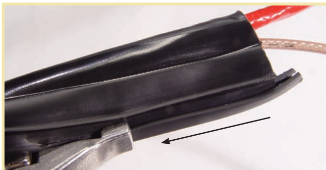
5. Carefully pull tool along slewing until closed.
