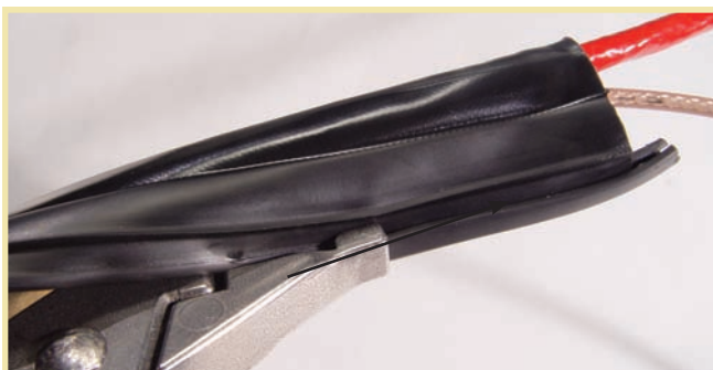
Use ZTZ-SP to disengage zip-track. Separate and slide tool up entire length to open.
