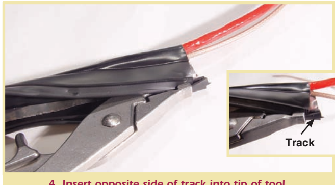
4. Insert opposite side of track into tip of tool. Make sure the tracks mate into each other.
