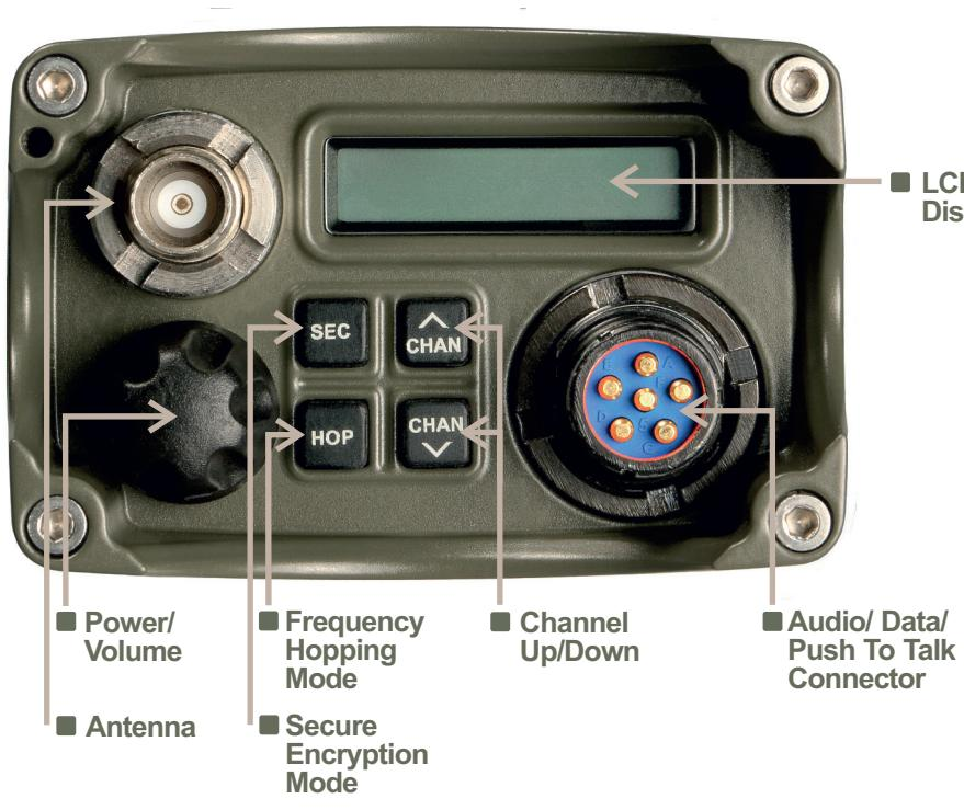
Advanced tactical handset for operation and field programming with U-229 style connector
