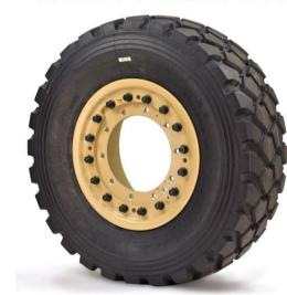
Multi piece wheels are designed for loads up to 5500kg in steel and aluminium. Designs are available as bolt together or three piece wheels with CTIS (central tyre inflation system) and RunFlat compatibility.
