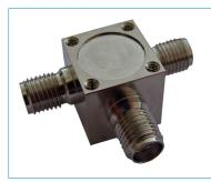
The I70105/A, I62104/A, I71121/A and I71121/A coaxial isolators were designed to be used for space-based frequency converters and receivers. Key requirements include electrical characteristics over a broad operating bandwidth, and exceptional EMC performance. These low power coaxial isolators can be supplied with any combination of SMA(m) and (f) connectors. Ports can be arranged with the load on any port. Note that these devices are also available as circulators.
